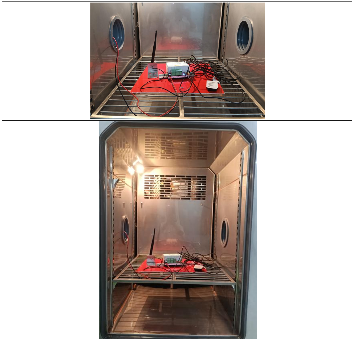
Figure 2: Cold Test Setup Photo
