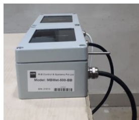
CORRECTS WAY (the cables to be downwards)
