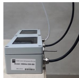
WRONG WAY (water can seep inside)
