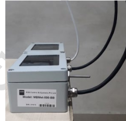
Fig-4.4: Proper way of securing the cables.
