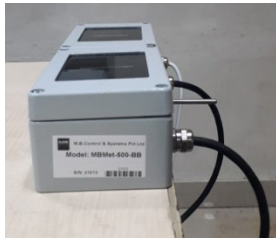
Fig-4.4: Proper way of securing the cables.
