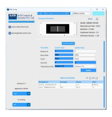
Configuration Software: "MB Config", a configuration software designed specially for configuration and trouble-shooting all MBMet Sensors. Users can download this Free to use software to a standard Laptop / PC and connect MBMet Sensors to it. All configuration settings, Modbus Frame Analysis, Heating Operation, Real-Time Data Viewing can be done seamlessly through this compact and powerful tool.
