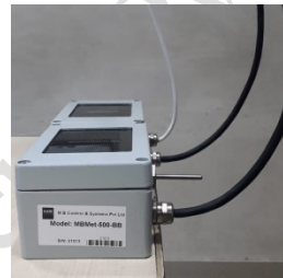
Fig-4.4: Proper way of securing the cables
