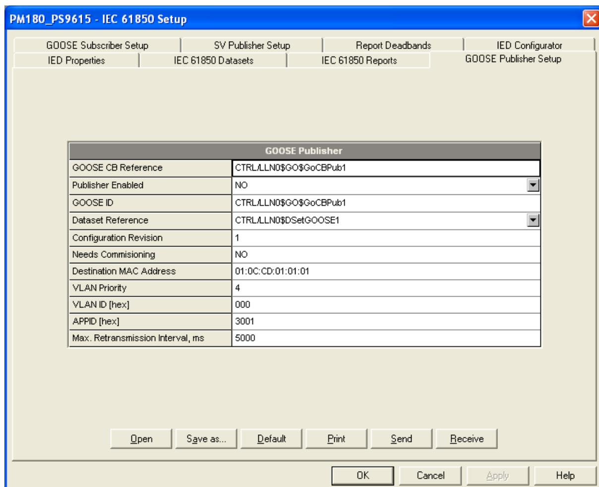
2. You can configure the destination MAC address, GOOSE ID, application ID and the maximum message retransmission interval for your application. You can also preset the configuration revision if needed. Other attributes are indicated for information only.
