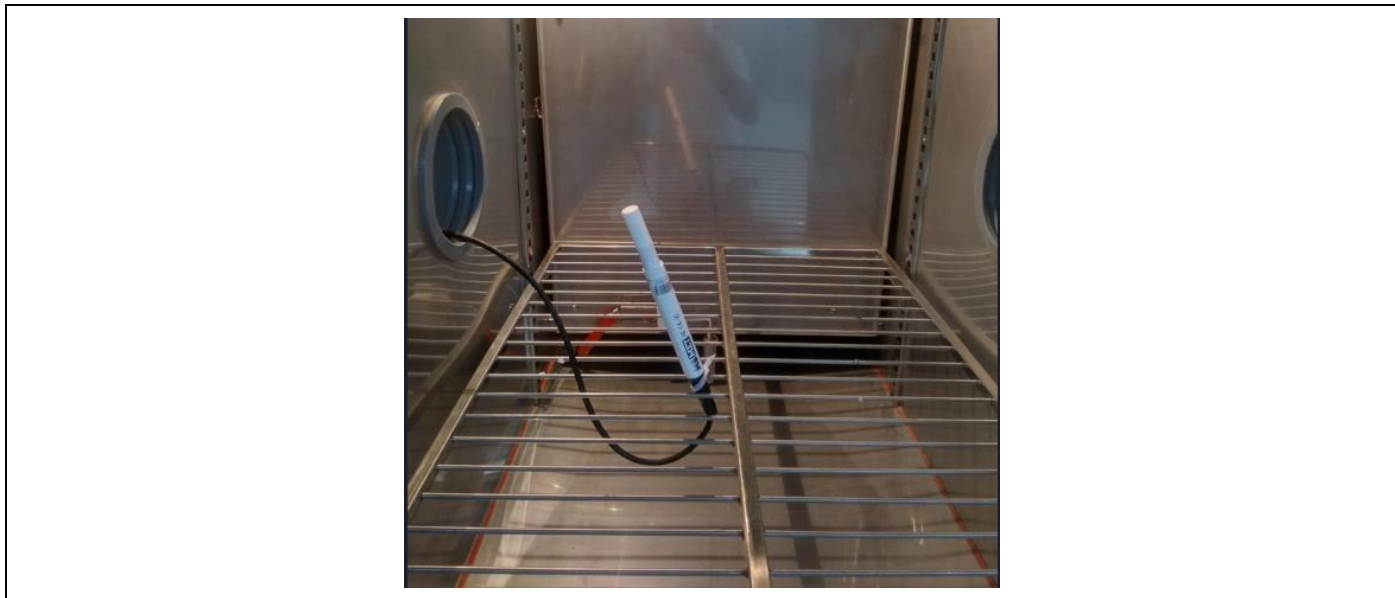
Figure 2: Damp Heat, Steady State Test Setup Photo
