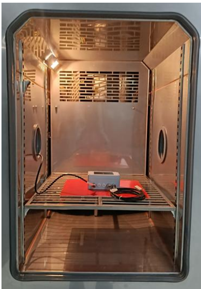
Figure 2: Dry Heat Test Setup Photo
