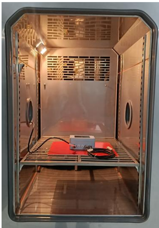
Figure 2: Damp Heat Steady State Test Setup Photo
