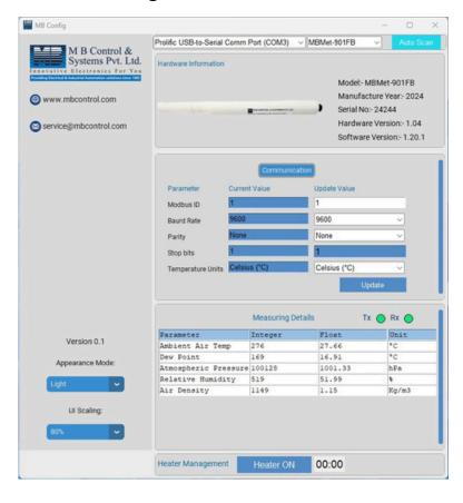
Configuration Software: "MB Config", a configuration software designed specially for configuration and trouble-shooting all MBMet Sensors. Users can download this Free to use software to a standard Laptop / PC and connect MBMet Sensors to it. All configuration settings, Modbus Frame Analysis, Heating Operation, Real-Time Data Viewing can be done seamlessly through this compact and powerful tool.
