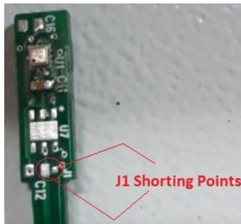
Fig: 6.3 Open top part of the sensor
