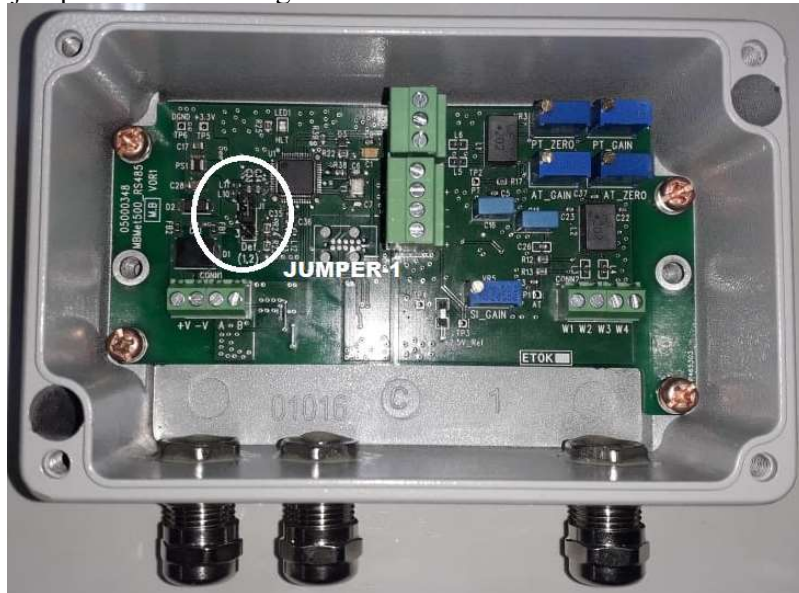
Fig – 7.3.1: Location of the Jumper 1
