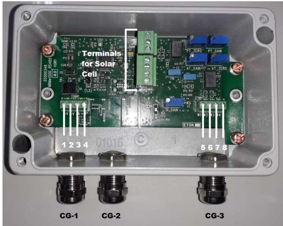
Picture – 5.1: Terminal Numbers of PCB
