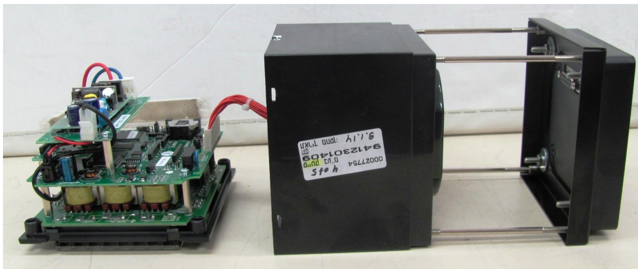
Fig. 11 PM175 - internal view
