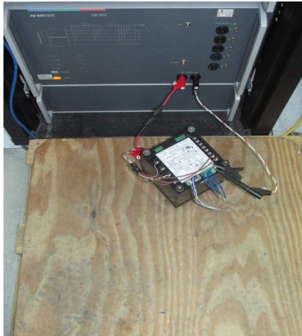
Test Picture 2: Surge on PM175
