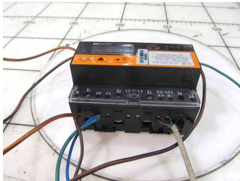
Picture #5 EM133 Radiated emission test setup
