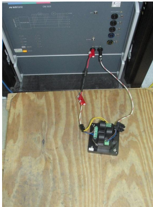
Test Picture 4: Surge on PM130EH Plus
