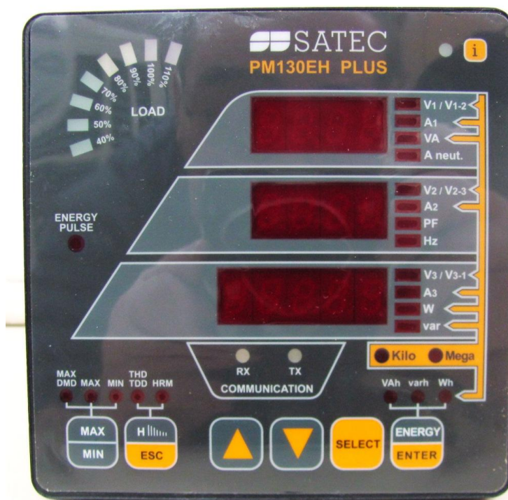
Fig. 7 PM130EH PLUS – front view
