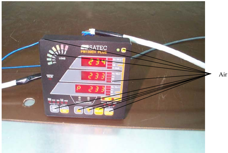
Figure 8. ESD Test Points
