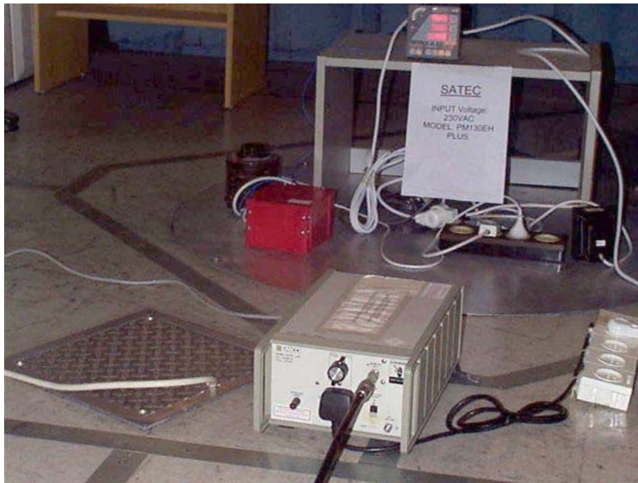
Figure 15. Conducted Emission Test
