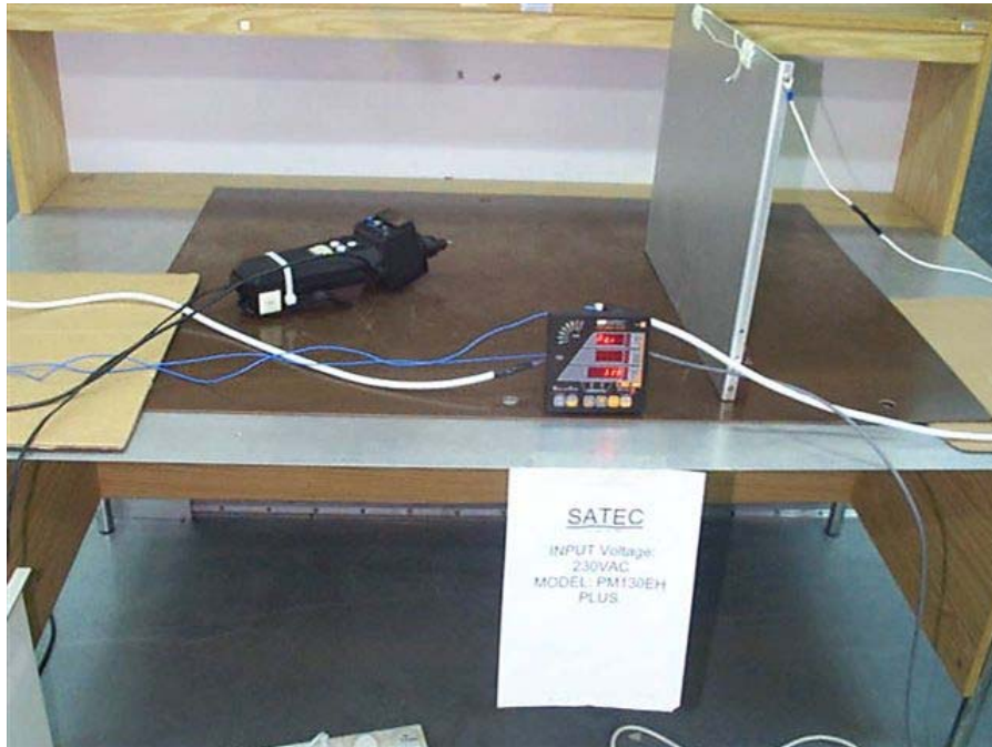
Figure 17. Immunity to Electrostatic Discharge Test
