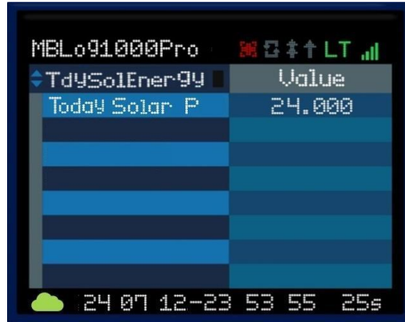
Figure-4.17: Today solar energy parameters display
