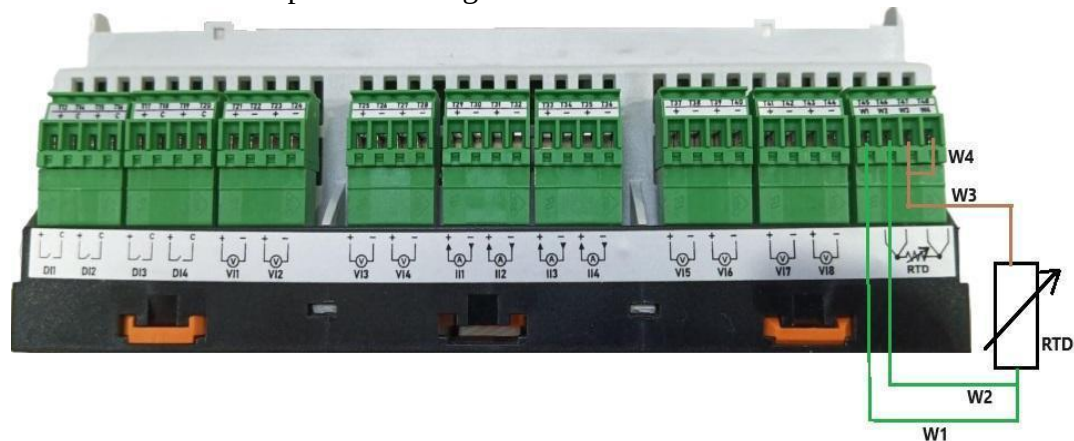
Figure-3.13.1: RTD input connections for three wire RTD sensor. (For Hardware version 5.00 and above)
