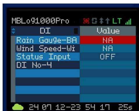
Figure-4.13: Digital inputs status and values
