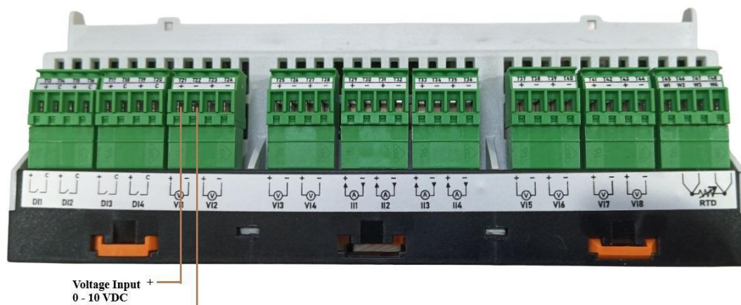
Figure-3.9: Measurement voltage (0-10VDC) input connections.
