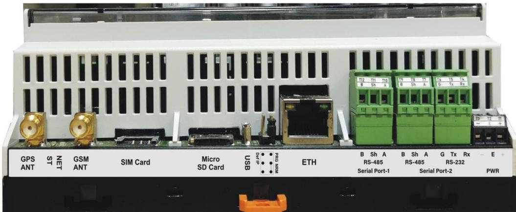
Figure-3.1.3: MBLogger communication port connectors and terminals (For Hardware version 3.11)
