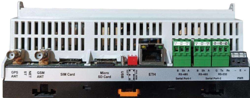
Figure-3.6: MLogger SD card slot.
