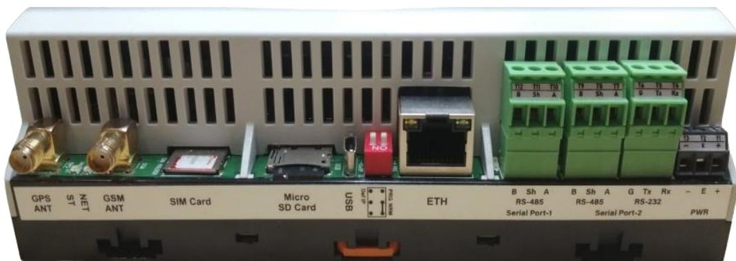
Figure-3.1.5: MBLogger communication port connectors and terminals (For Hardware version 5.11)
