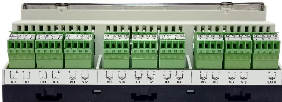
Figure-3.1.2: MLogger Signal input terminals (For Hardware version 2.11)
