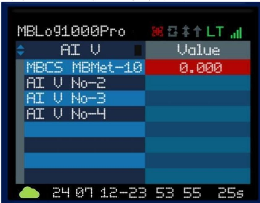
Figure-4.9: Measured voltage channel values
