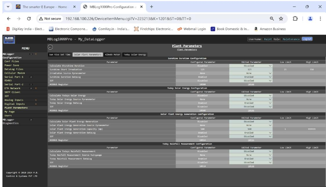
Figure-6.21.2: Configure Solar Plant Parameters.
