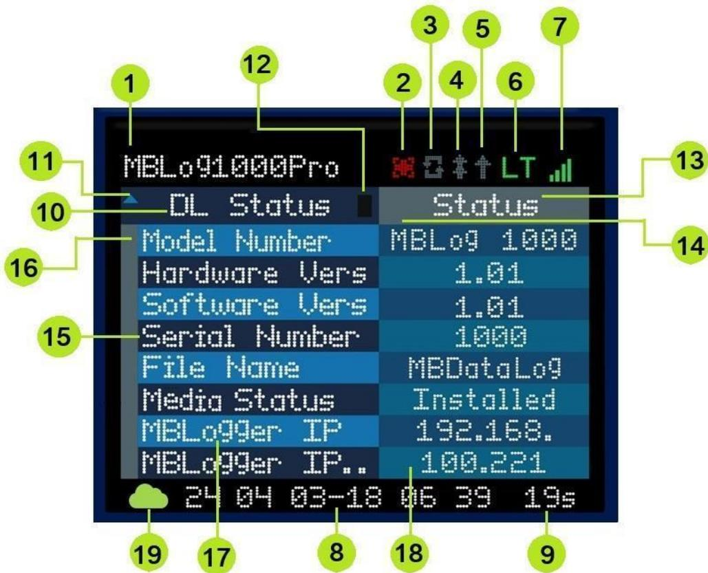
Figure-4.3: Datalogger OLED
