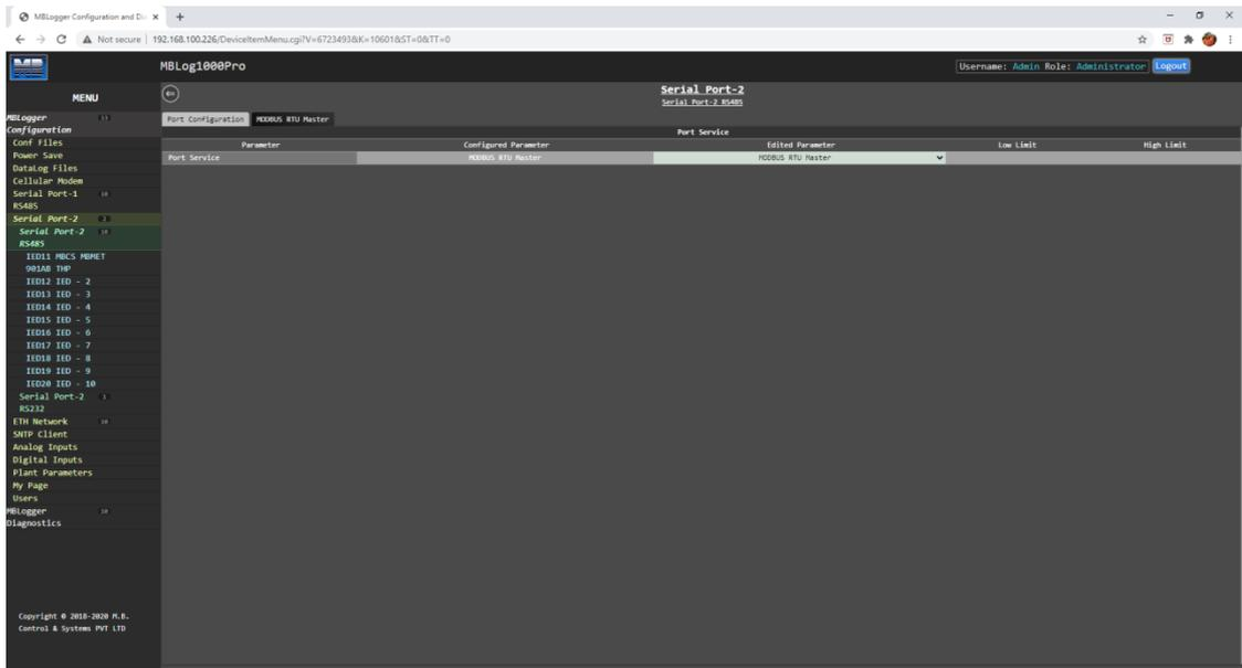
Figure-6.10.1: Configuration of serial port-2 RS485.
