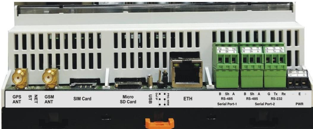
Figure-3.1.3: MBLlogger communication port connectors and terminals (For Hardware version 3.11)
