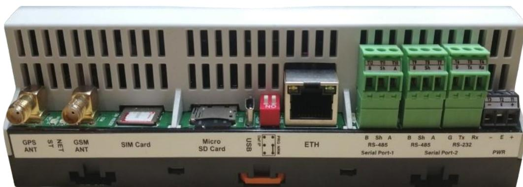
Figure-3.1.5: MBLlogger communication port connectors and terminals (For Hardware version 5.11)
