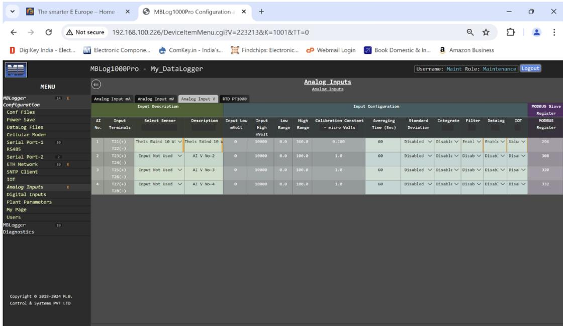
Figure-6.16.3: Configuration of Voltage input channels.
