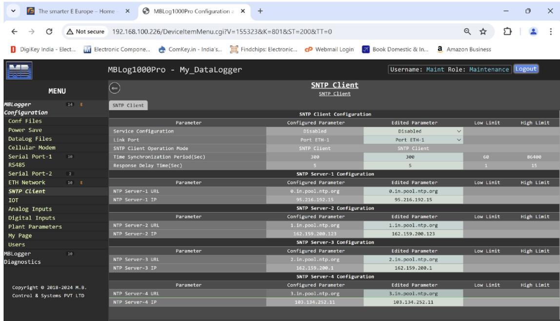
Figure-6.14: Configuration of SNTP client.
