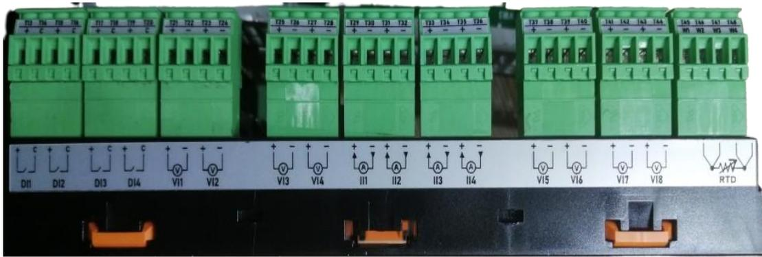
Figure-3.1.6: MBLogger signal input terminals (For Hardware version 5.11)
