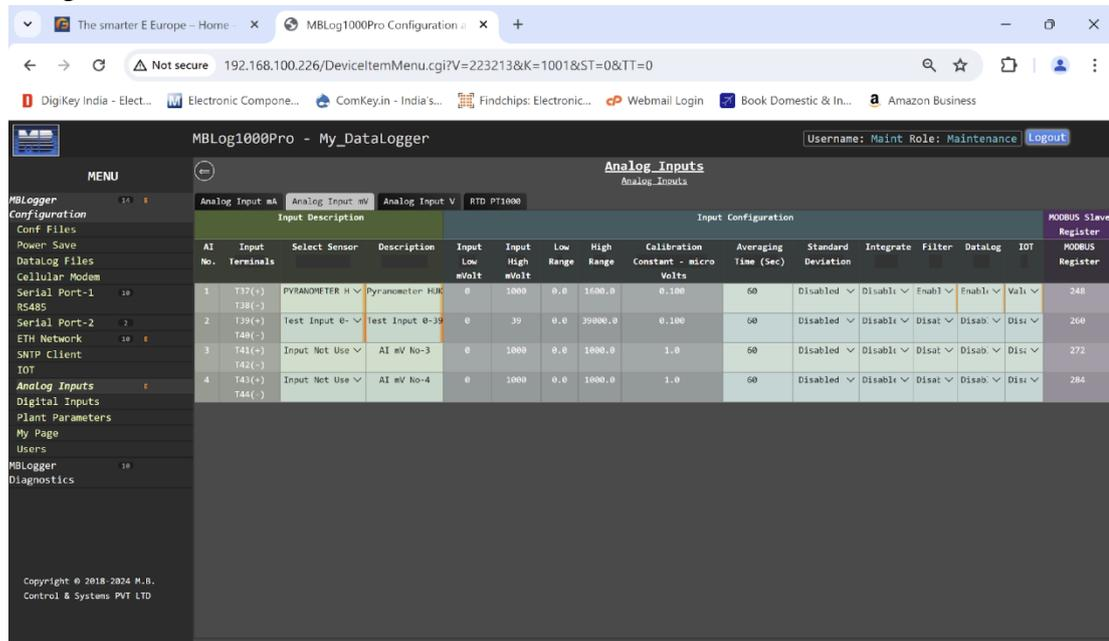
Figure-6.16.2: Configuration of mV input channels.
