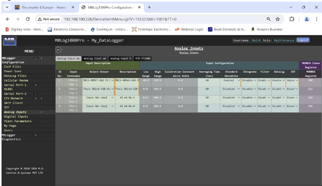
Figure-6.16.1: Configuration of mA input channels.
