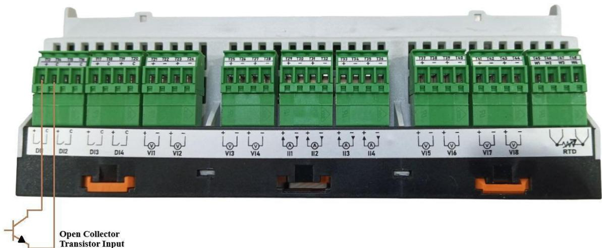
Figure-3.8.2: Digital input connections for open collector transistor inputs.
