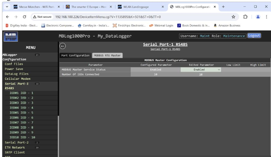
Figure-6.9: Configuration of serial port-1 RS485.
