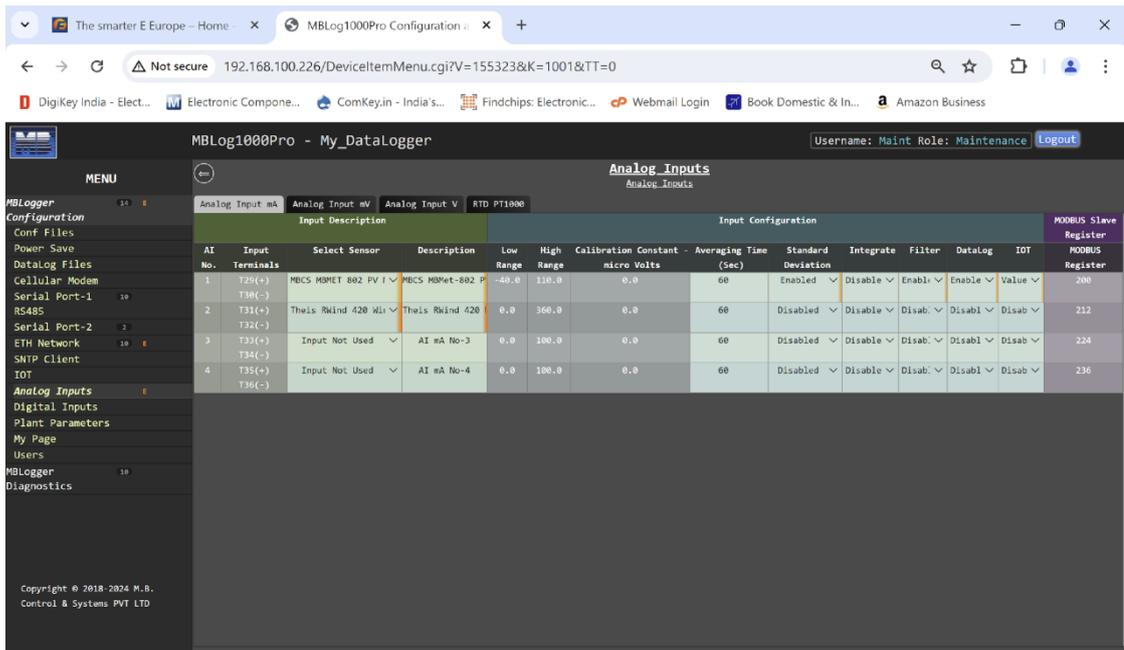
Figure-6.16: Configuration of analog input channels.
