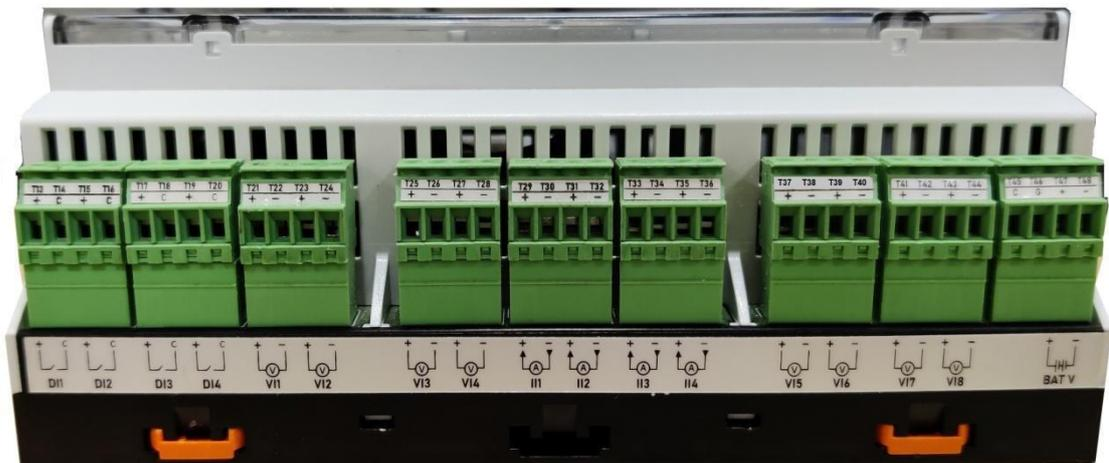
Figure-3.1.4: MBLlogger signal input terminals (For Hardware version 3.11)
