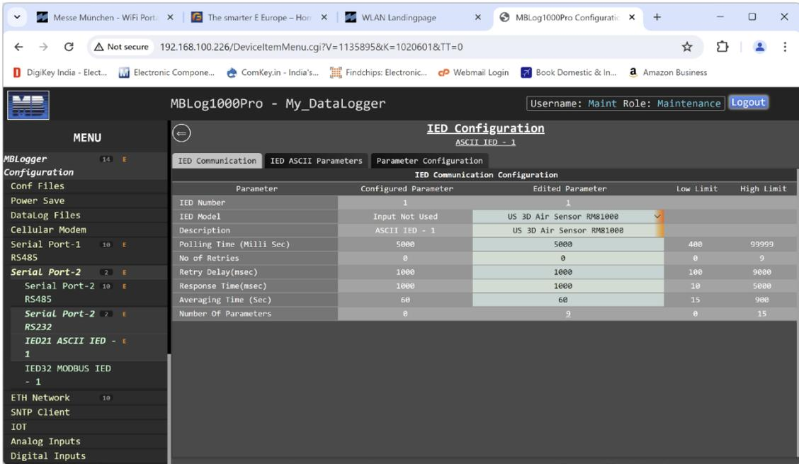
Figure-6.13.1: Configuration of ASCII IED communication parameters.
