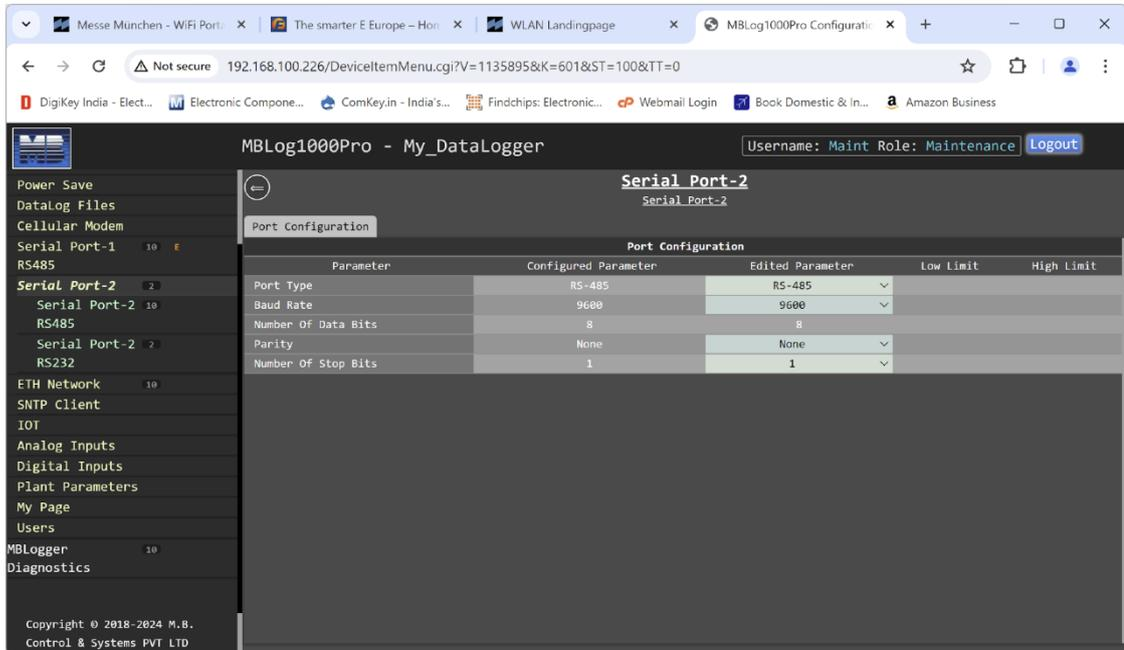
Figure-6.10: Configuration of serial port-2.
