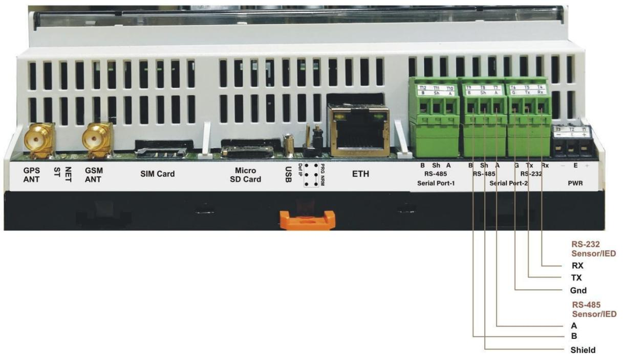
Figure-3.4: MLogger serial port-2 (RS485 or RS232) connections.
