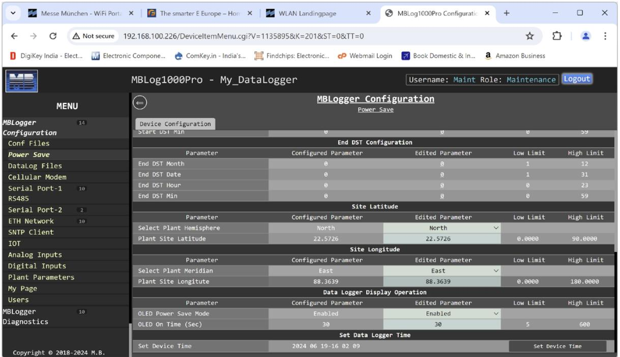
Figure-6.4.3: Configuration of datalogger OLED power save parameters.
