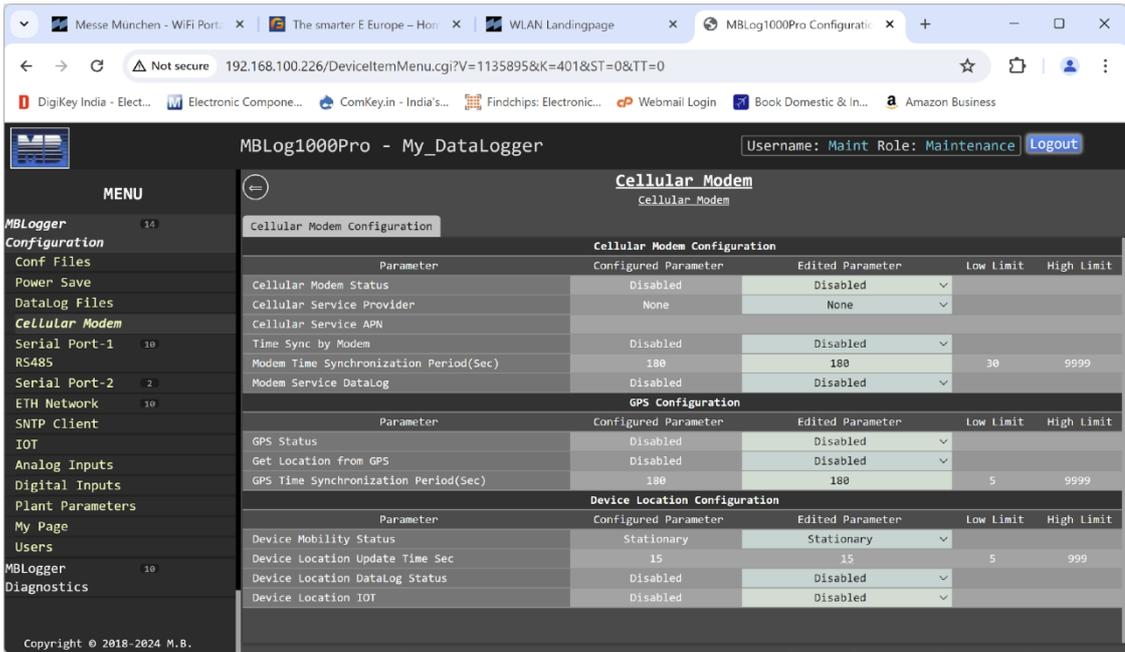
Figure-6.6: Configuration of internal cellular modem.
