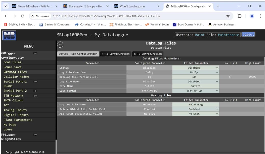
Figure-6.5: Configuration of data log file operations.
