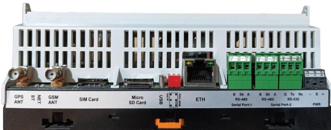
Figure-3.7: MLogger internal modem.
