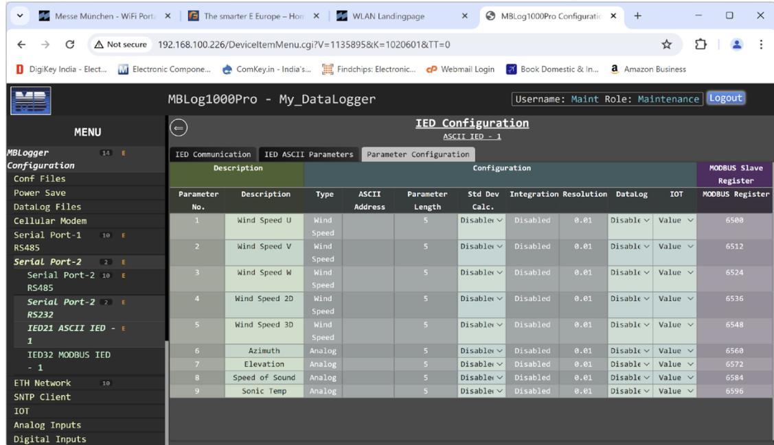
Figure-6.13.3: Configuration of ASCII IED read parameters.
