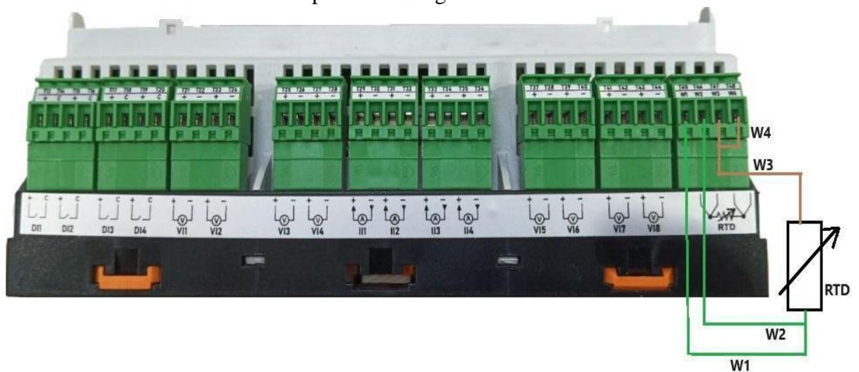
Figure-3.13.1: RTD input connections for three wire RTD sensor.
