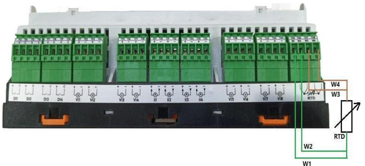
Figure-3.13.1: RTD input connections for four wire RTD sensor.
