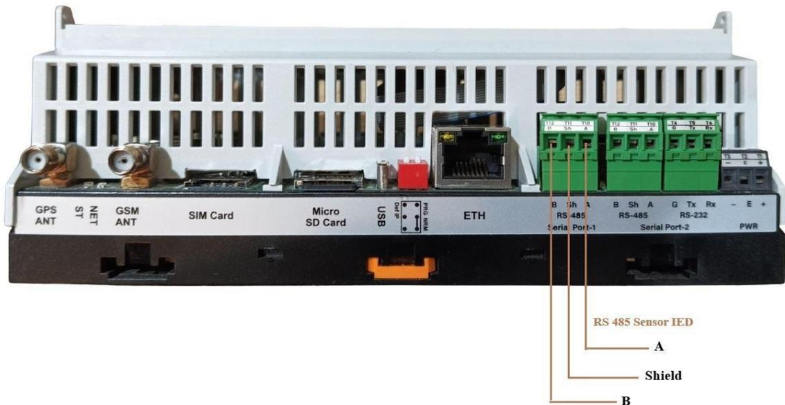
Figure-3.3: MLogger serial port-1 (RS485) connections.
