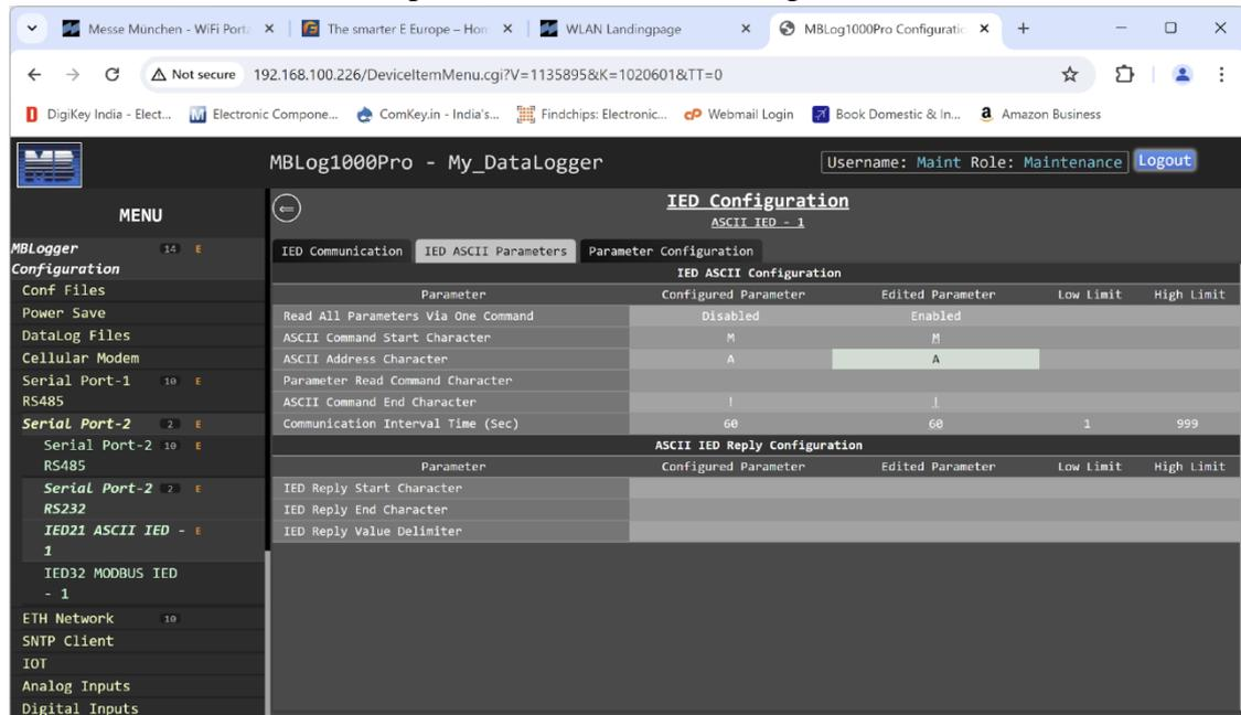
Figure-6.13.2: Configuration of IED ASCII communication parameters.
