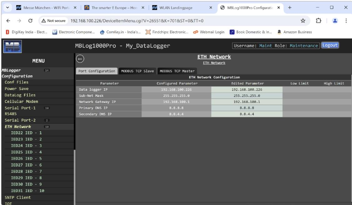
Figure-6.11: Configuration of datalogger ETH network.
