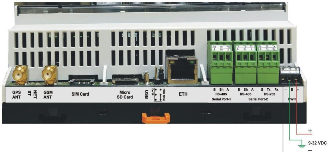
Figure-3.2: MBLogger power supply connections.
