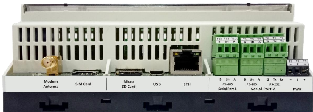
Figure-3.1.1: MBLogger communication ports and terminals (For Hardware version 2.11)
