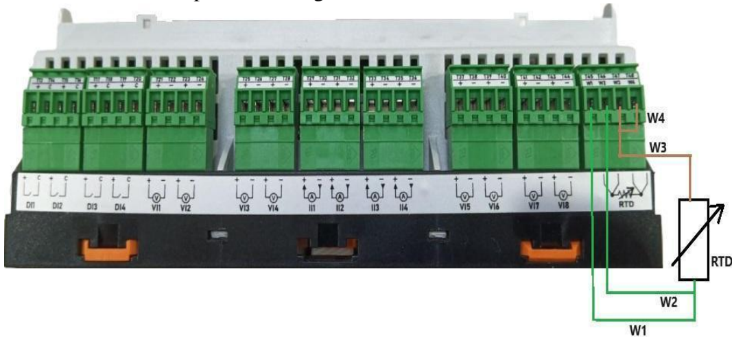
Figure-3.13.1: RTD input connections for three wire RTD sensor. (For Hardware version 5.00 and above)
