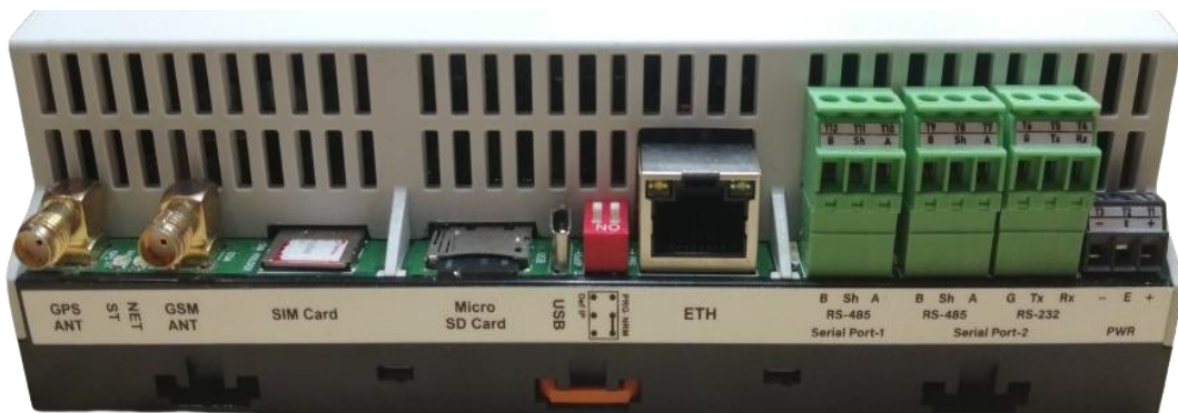
Figure-3.1.4: MBLLogger communication port and terminals (For Hardware version 5.11)
