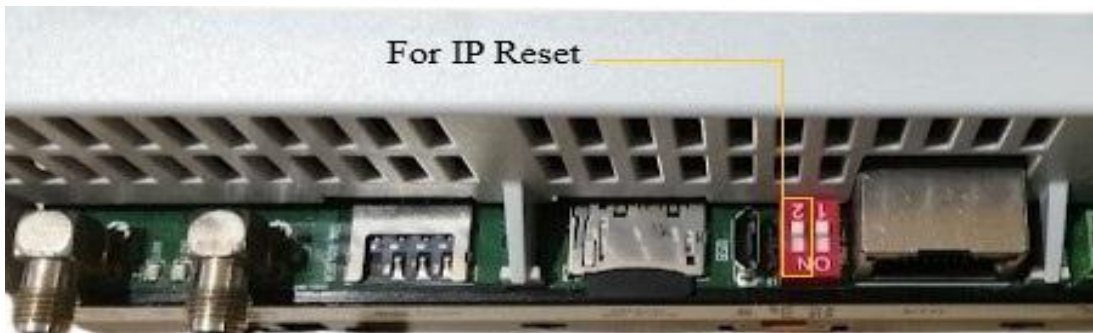
Figure -5.2: Dip Switches for setting default IP address in the datalogger HW version 5.1 and above.
