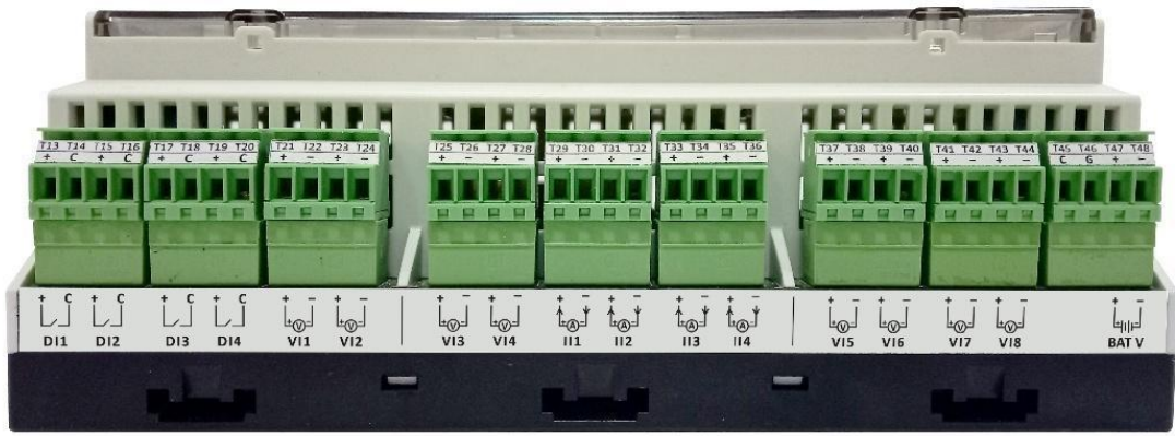
Figure-3.1.2: MBLLogger Signal input terminals (For Hardware version 2.11 and 3.11)
