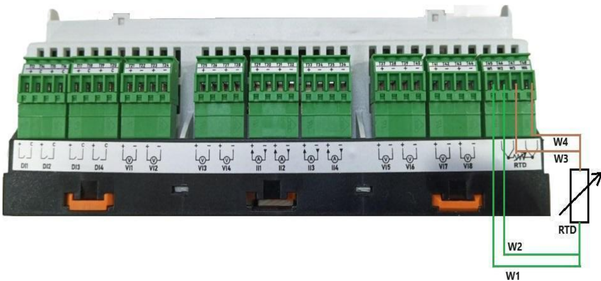
Figure-3.13.1: RTD input connections for four wire RTD sensor. (For Hardware version 5.00 and above)
