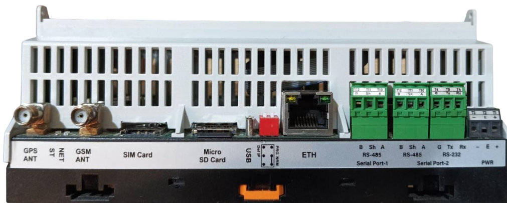
Figure-3.6: MBLogger SD card slot.
