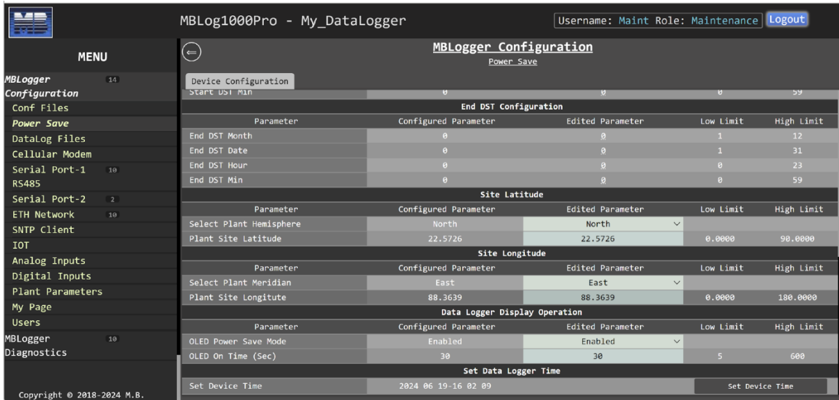
Figure-6.4.3: Configuration of datalogger OLED power save parameters.
