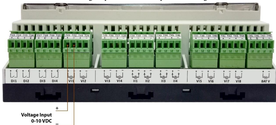
Figure-3.9: Measurement voltage (0-10VDC) input connections.
