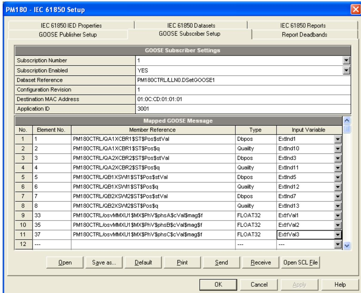
Select compatible input variables to which dataset elements will be mapped in the device. See the table below for allowable mapping options depending on the basic variable type.
