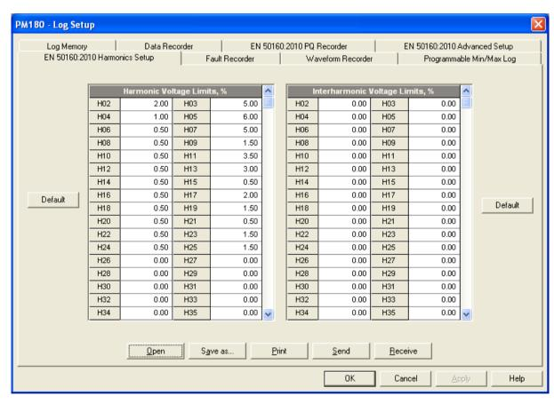
The default settings contain values of individual harmonic voltages specified by the standard for low-voltage networks. To automatically pre-set compliance limits for a medium-voltage or high-voltage network, ensure that the nominal voltage and PT ratio settings in your device's Basic Setup match the actual network characteristics, and then click on the Default button.
