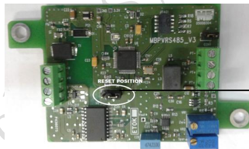
Fig – 8.3: Jumper position (for factory resetting)
