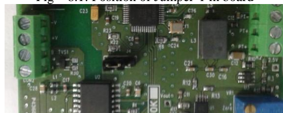
Fig – 8.2: Jumper position (factory setting)
