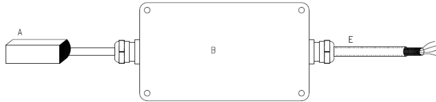
Fig 1.1 –PV Module Surface Temperature transducer (RS-485)
