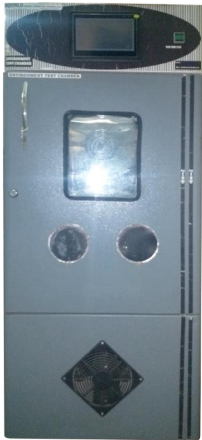
Environment Controlled Chamber
