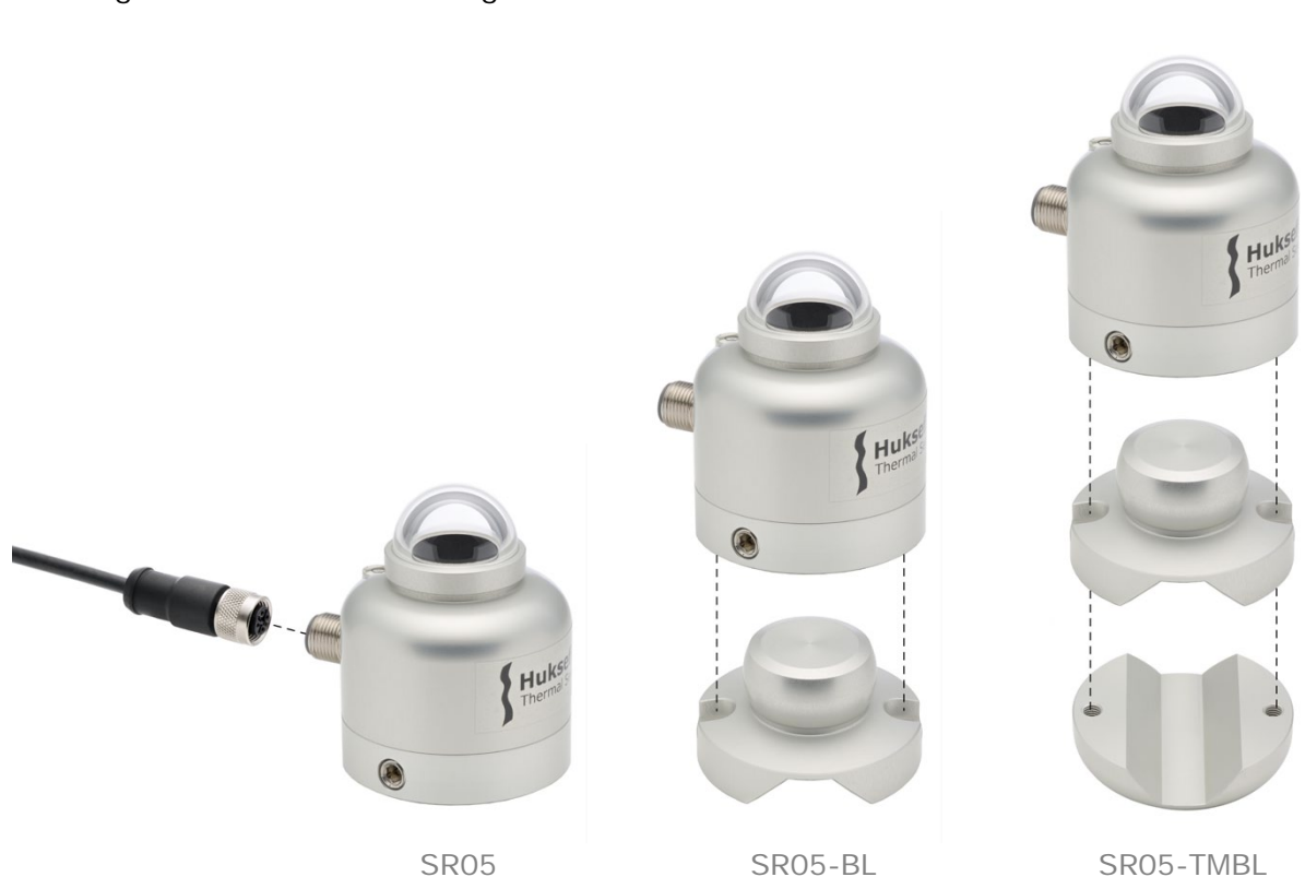
Figure 5.2.1 From left to right: SR05 in its standard configuration with 3 metre cable; with optional ball levelling for easy mounting and levelling on a (non-)horizontal surface; with optional ball levelling and tube mount for easy installation on a 25 to 40 mm diameter tube. Mounting bolts are included with the ball levelling and / or tube mount.
