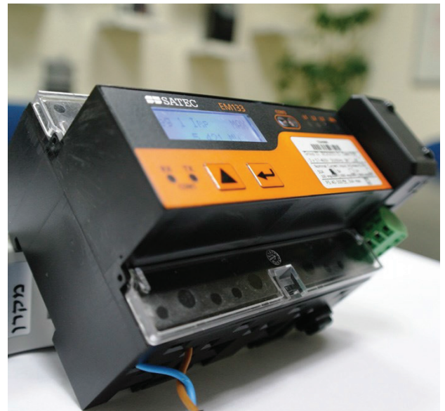
SATEC EM133 with Cellular Modem
