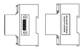
Figure 2-4. EM13X Series module connector location
