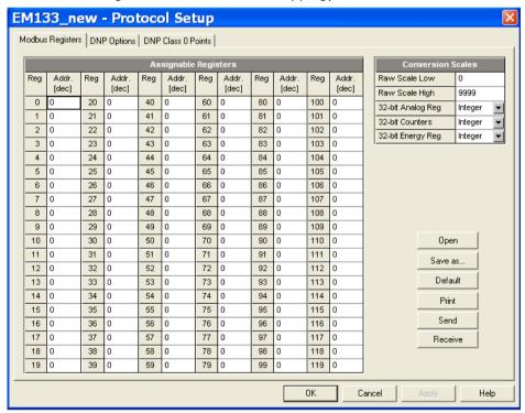
Figure 5-21: Protocol Setup Dialog Box - MODBUS Registers Tab
