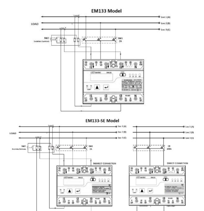
Figure 2-12 3-Wire 2-Element Delta Direct Connection Using 2 CTs (Wiring Mode = 3dir2)
