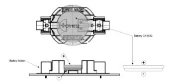
Figure 2-7 EM13X Series Battery Replacement
