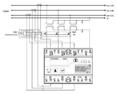
Figure 2-14 4-Wire Wye 3-Element Connection Using 3 PTs, 3 CTs (Wiring Mode = 4LL3 or 4Ln3)
