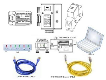
Figure 2-23 COM2 Ethernet Connection
