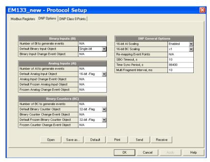
Figure 5-22: Protocol Setup Dialog Box - DNP Options Tab
