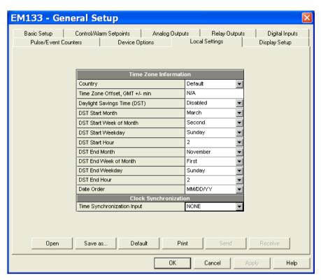
Figure 5-14: General Setup Dialog Box - Local Settings Tab
