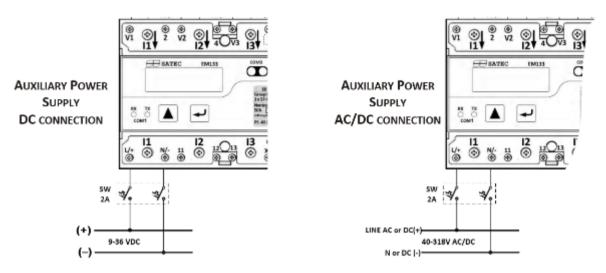
Figure 2-8 EM13X Series Auxiliary Power Supply connection
