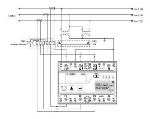
Figure 2-17 3-Wire 2½-Element Open Delta Connection Using 2 PTs, 3 CTs (Wiring Mode = 30P3)
