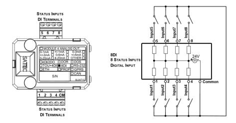
Figure 2-13 8 DI - Digital Input Connection
