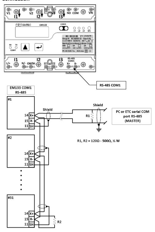
Figure 2-19 COM1 RS-485 2-Wire Connection
