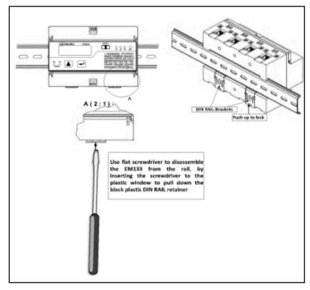
Mounting the EM13X Series on DIN-Rail
