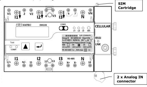
Figure 2-28b COM2 2G/3G+2AI DIN Rail module Connection
