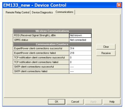
Figure 6-5: Device Control Dialog Box - Communications Tab
