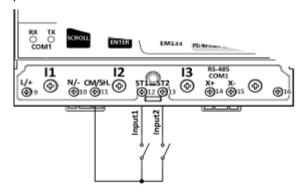
Figure 2-9 EM13X Series Digital Input connections
