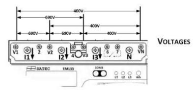
Figure 2-9EM13X Series (with Aux. Power Supply) measured Voltage connections
