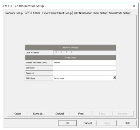
Figure 5-3: Communication Setup Dialog Box - GPRS Setup Tab
