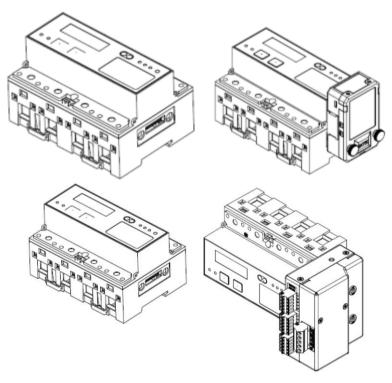
Figure 2-5. EM13X Series module assembly
