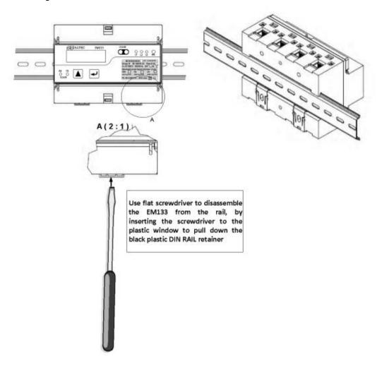
Figure 2-3. EM13X Series DIN Rail Mounting
