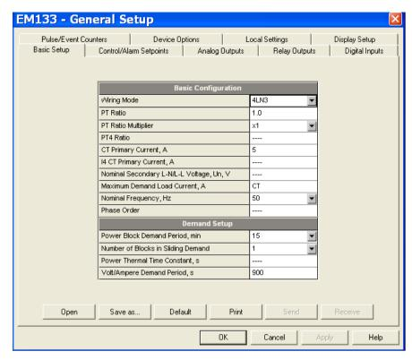
Figure 5-6: General Setup Dialog Box - Basic Setup Tab
