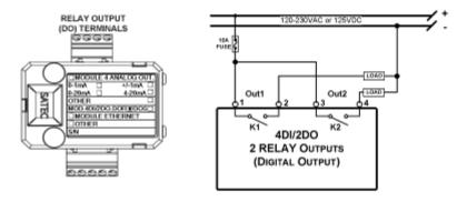
Figure 2-11 Relay Output Connection
