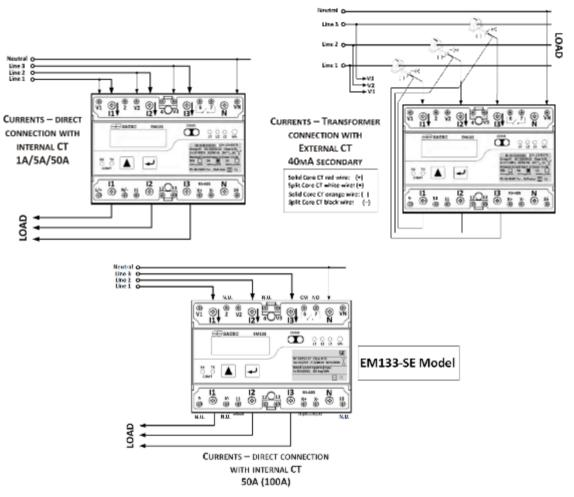
Figure 2-11 EM13X Series measured Current connections
