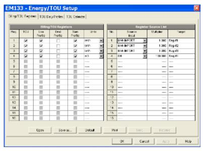
Figure 5-16: Energy/TOU Setup Dialog Box - Billing/TOU Registers tab
