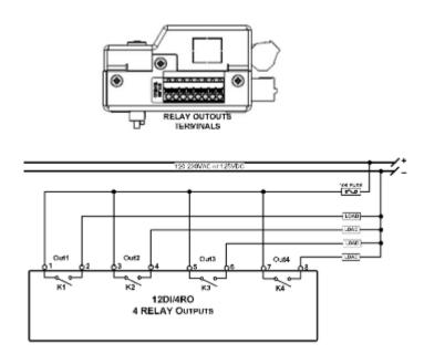
Figure 2-15 Relay Output Connection
