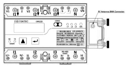
Figure 2-30 COM2 RF module Connection
