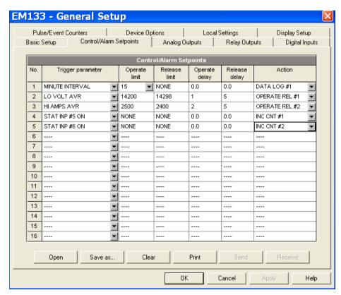
Figure 5-12: General Setup Dialog Box - Control/Alarm Setpoints Tab
