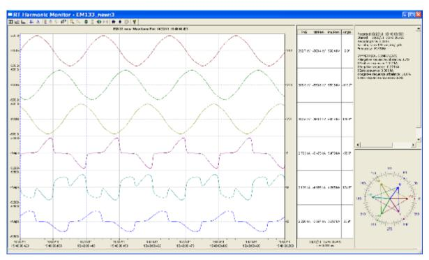
Figure 7-6: RT Harmonic Monitor – Synthesized Waveforms
