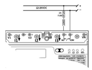
Figure 2-8 EM13X Series Relay output connection
