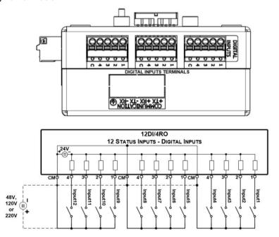
Figure 2-16 12 Digital Input Connection
