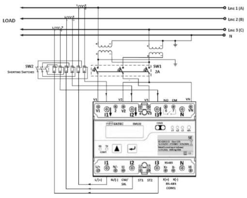
Figure 2-19 3-Wire 2½-Element Broken Delta Connection Using 2 PTs, 3 CTs (Wiring Mode = 3bLn3 or 3bLL3)
