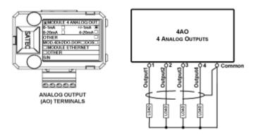
Figure 2-18 Analog Output Connection
