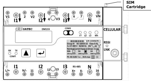
Figure 2-29b COM2 2G/3G/4G DIN Rail module Connection
