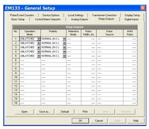
Figure 5-9: General Setup Dialog Box - Relay Outputs Tab
