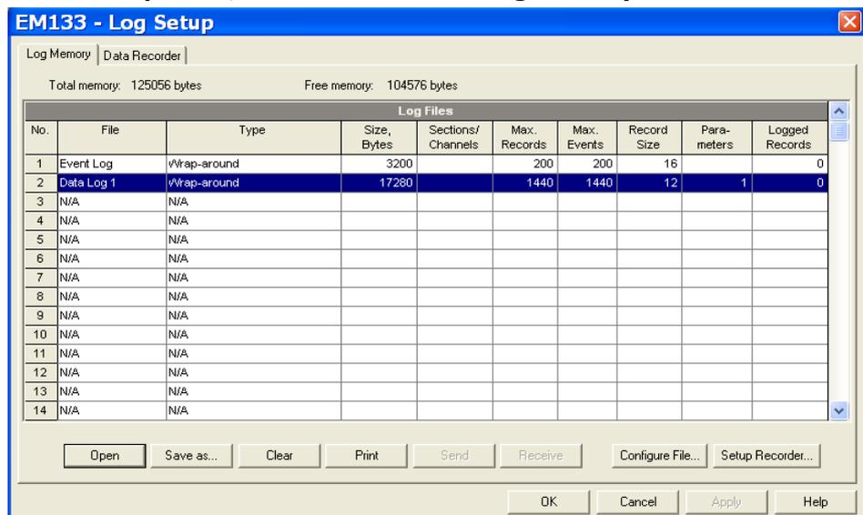
**Figure 5-19: Log Setup Dialog Box – Log Memory Tab**
