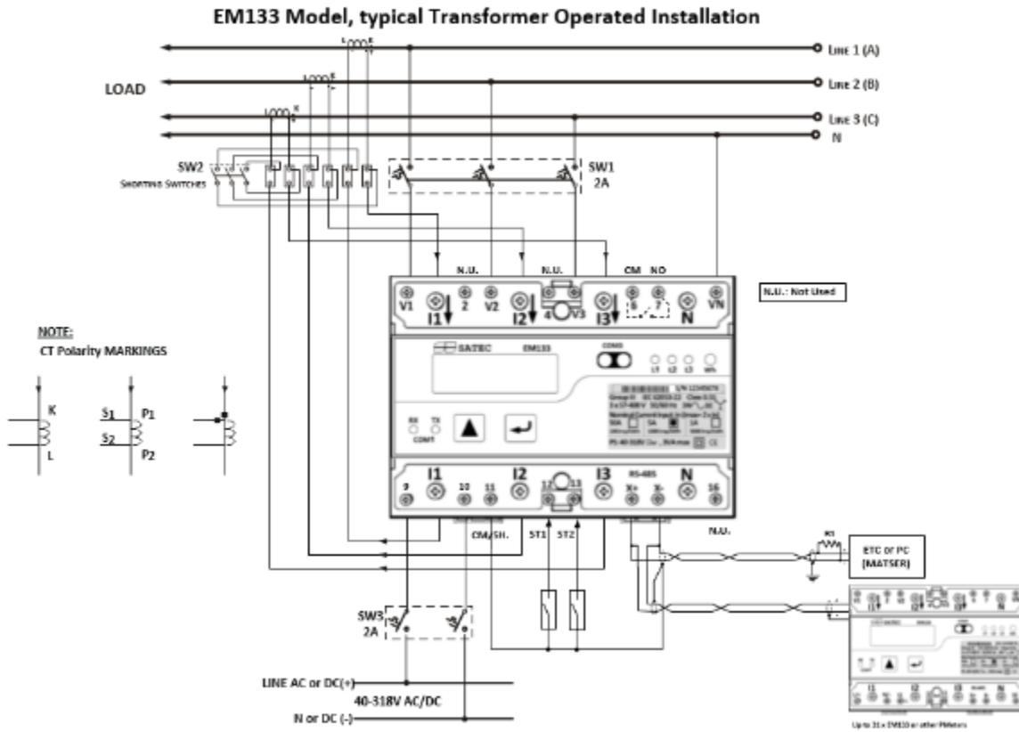
Figure 2-6a Typical Installation Diagram with Auxiliary Power Supply
