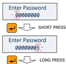
The setup menus are secured by 8-digit user passwords. Every time you enter programming mode, you are prompted for a correct password. The meter is primarily shipped with all passwords preset to 9 at the factory.
