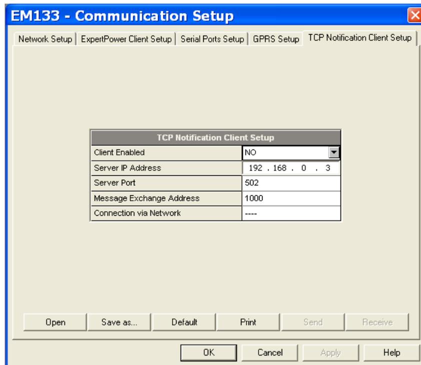
**Figure 5-5: TCP Notification Client Setup Tab**
