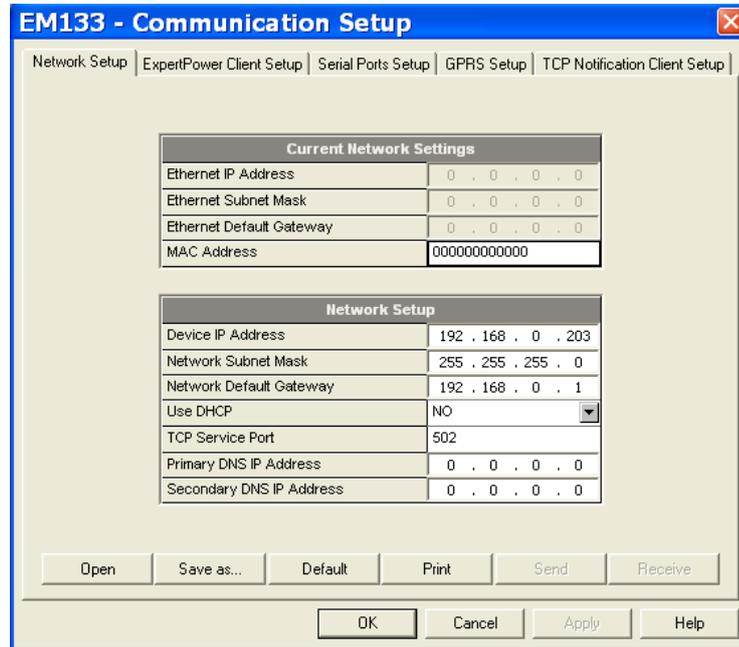
**Figure 5-2: Communication Setup Dialog Box – Network Setup Tab**
