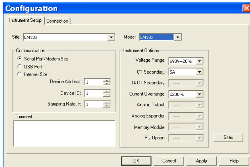
**Figure 4-1: Configuration Dialog Box – Instrument Setup Tab**
