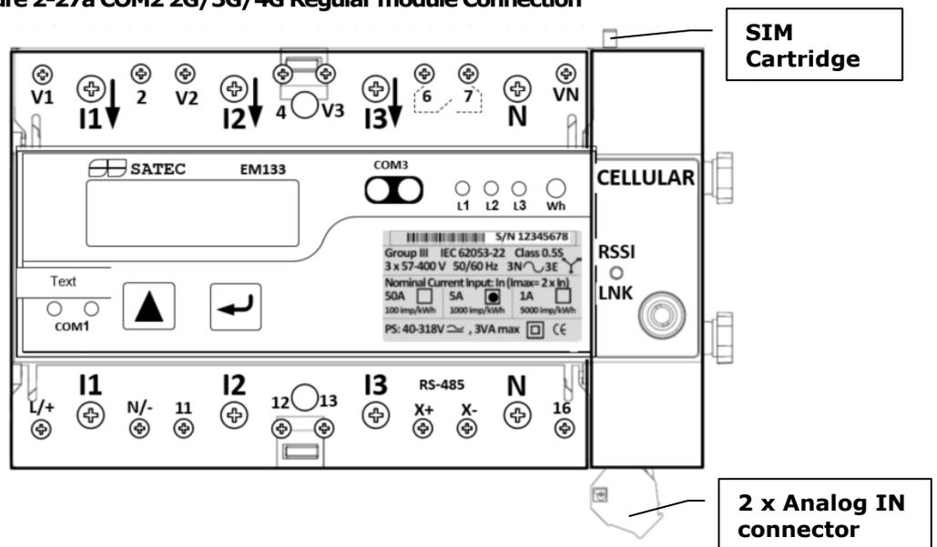
**Figure 2-28b COM2 2G/3G+2AI DIN Rail module Connection**
