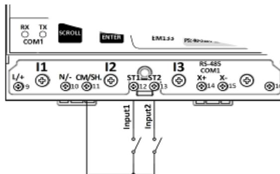
Figure 2-9 EM13X Series Digital Input connections
