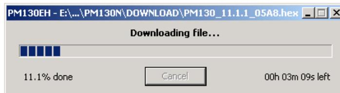
After upgrading firmware is completed, the meter restarts, so communications can be temporarily lost. You may need to wait a short duration until PAS restores a connection with your device.
