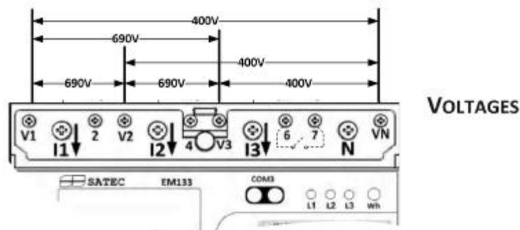
Figure 2-9 EM13X Series (with Aux. Power Supply) measured Voltage connections
