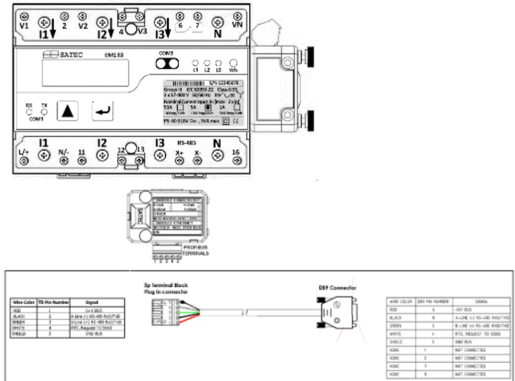
Figure 2-24 COM2 PROFIBUS Connection
