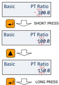
Whenever a numeric value is to be changed, use a short press on the SELECT/ENTER button to highlight a desired digit, and then use the SCROLL button to change the value of the highlighted digit. A highlighted digit appears in inverted color. If you missed a digit, just continue moving through the rest of digits until you reach the desired place.
