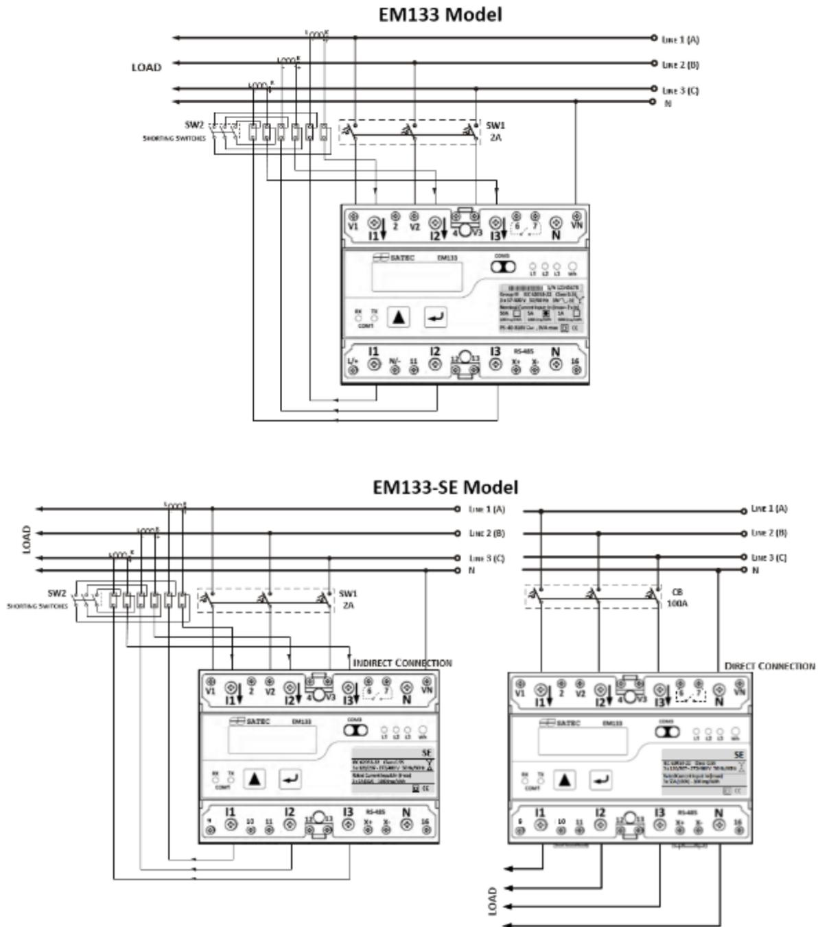
Figure 2-13 4-Wire Wye 3-Element Direct Connection Using 3 CTs (Wiring Mode = 4LL3 or 4Ln3)
