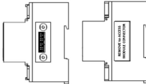
Figure 2-4. EM13X Series module connector location
