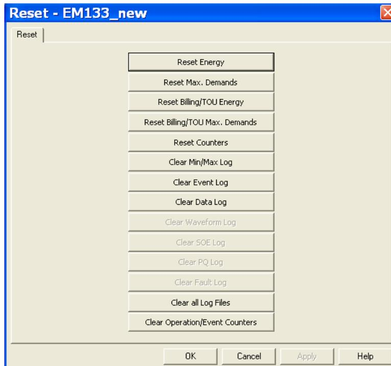
**Figure 6-1: Reset Dialog****To reset the desired values or files:**
