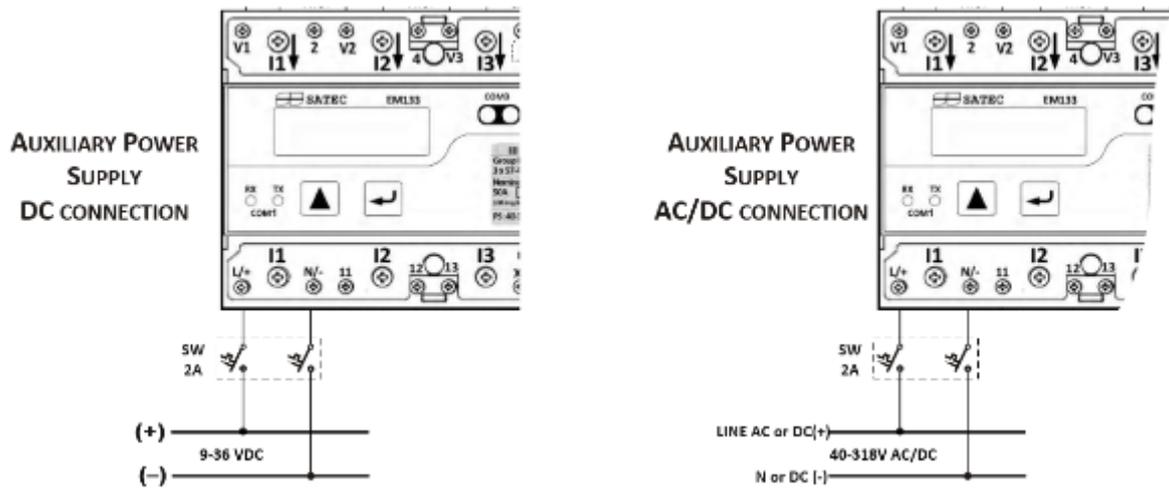
**Figure 2-8 EM13X Series Auxiliary Power Supply connection**
