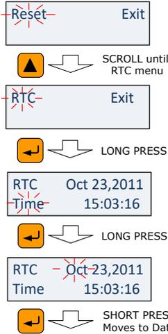
When in RTC setup menu, applying a LONG PRESS on the **SELECT/ENTER** button will display the **Time/Date** screen while **Time** willflash. Another LONG PRESS on **SELECT/ENTER** button will flash the actual hour to be changed using **SCROLL** button
