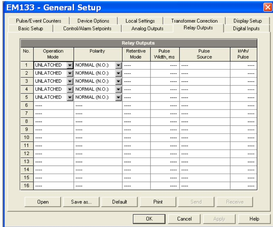
Figure 5-9: General Setup Dialog Box – Relay Outputs Tab
