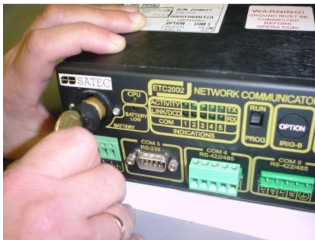
Figure 7-4 Insertion of New Battery
