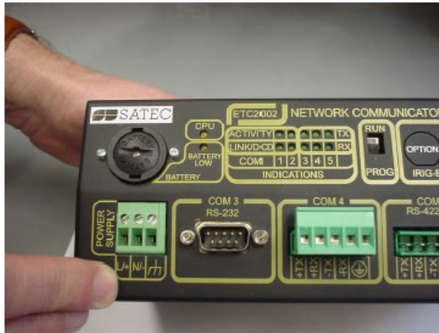
Figure 7-1 Battery Housing Location of the Panel
