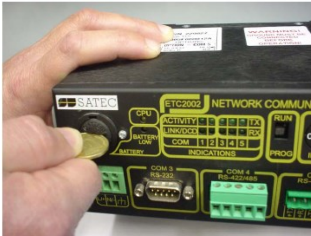
Figure 7-2 Battery Housing Cover Removal
