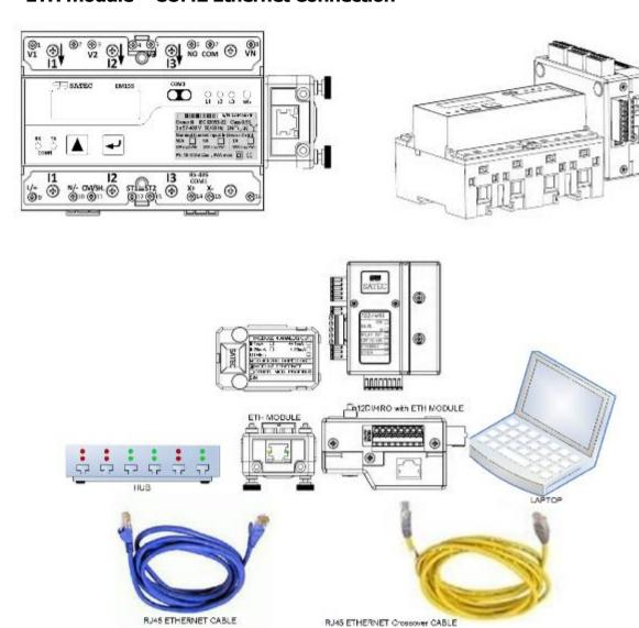
Figure 2-20 COM2 Ethernet Connection
