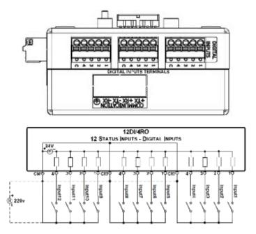
Figure 2-16 12 Digital Input Connection
