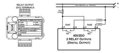
Figure 2-11 Relay Output Connection
