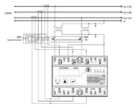
This configuration provides accurate power measurements only if the voltages are balanced.
