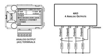
Figure 2-18 Analog Output Connection
