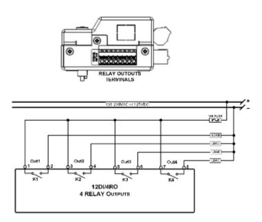
Figure 2-15 Relay Output Connection
