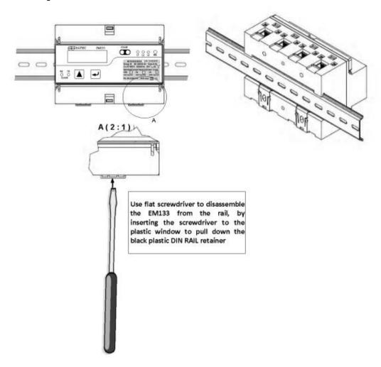
Figure 2-3. EM13X Series DIN Rail Mounting
