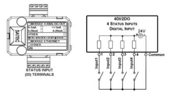
Figure 2-12 4 DI/2DO - Digital Input Connection
