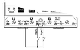
Figure 2-9 EM13X Series Digital Input connections
