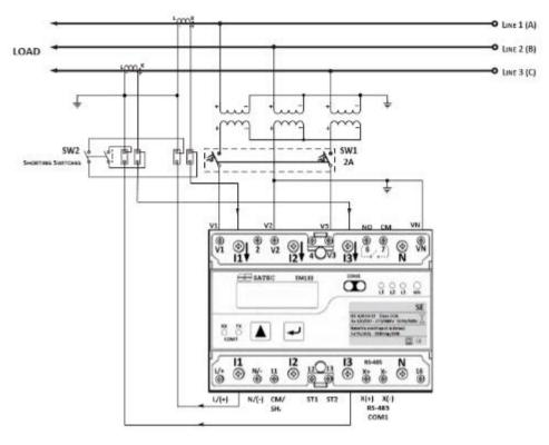
Figure 2-15b 3-Wire 2-Element Open Delta Connection Using 3 PTs, 2 CTs (Wiring Mode = 30P2)
