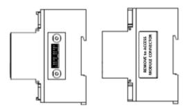
Figure 2-4. EM13X Series module connector location
