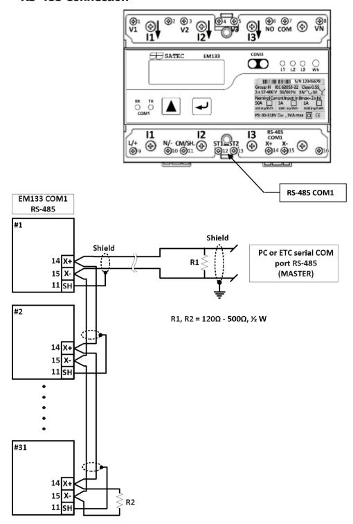
Figure 2-19 COM1 RS-485 2-Wire Connection
