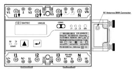
Figure 2-25 COM2 RF module Connection
