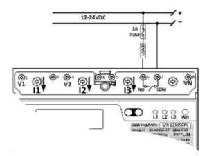
Figure 2-8 EM13X Series Relay output connection
