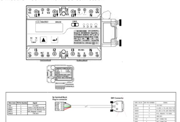
Figure 2-21 COM2 PROFIBUS Connection
